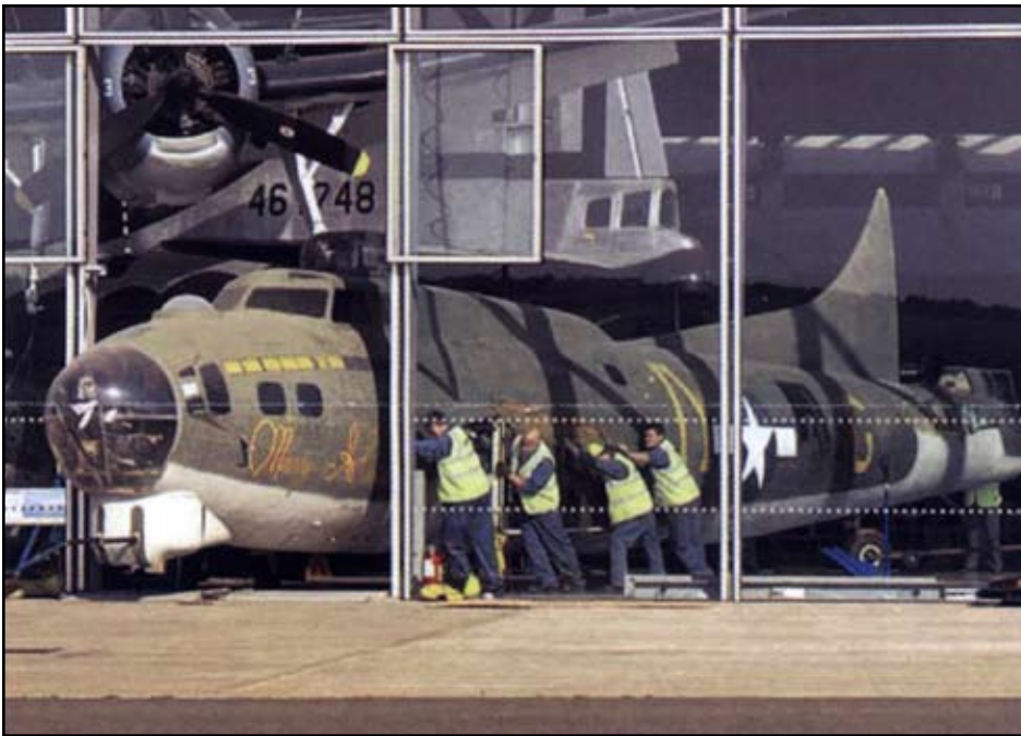
THIS UNUSUAL PHOTO shows workmen rolling the B-17, Mary Alice, out of the American Air Museum in Britain. The wings were detached in order to move the Fortress out of the fire exit, saving the removal of the huge plate glass windows. Renovation and a new paint job will take place at another facility on the Air Museum's grounds in Duxford, England.
